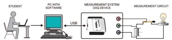
Each experiment is performed by starting the soft ware in *LabVIEW* that controls the measurement process and records the results of the measurements.
