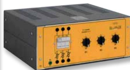
Carico resistivo – Resistive load
