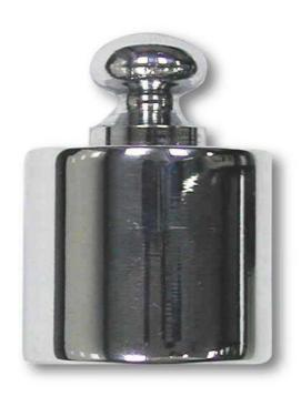
The 200 gram standard weight that use for executing the self-calibration function.
